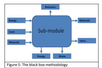
The flows in and out of sub-module will be defined (where needed) in three values, the minimum, set point and maximum value possible. These values will be used as variable parameters within the biogas simulator. The modular approach, together with the input output analysis is a transparent method for dynamic modelling, with the added advantage of expandability with a theoretically unlimited amount of new sub-modules.
