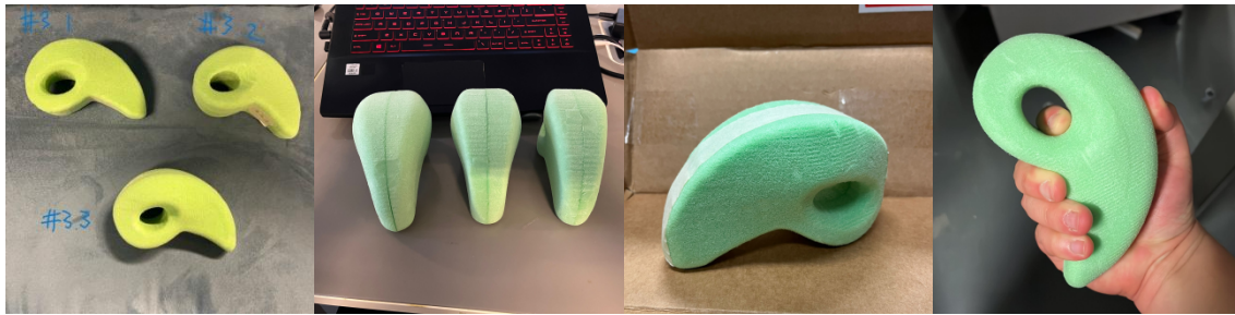
Fig.2. Foam models testing the design form and identifying contact points.
