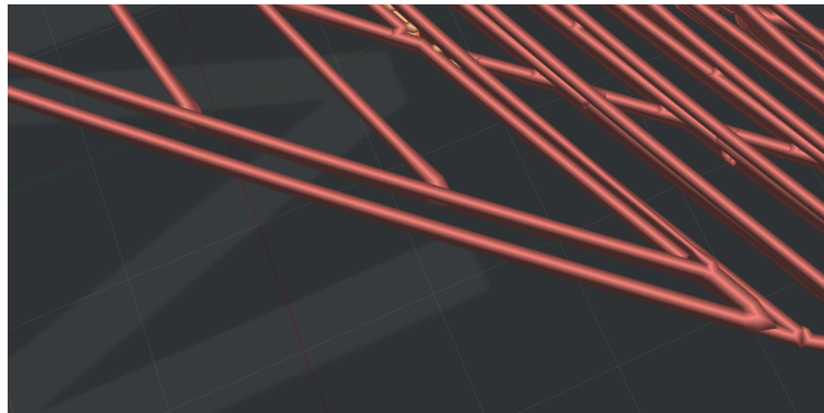
Image 4. Channel for wire insertion as seen in slicing software. (Source: author)
