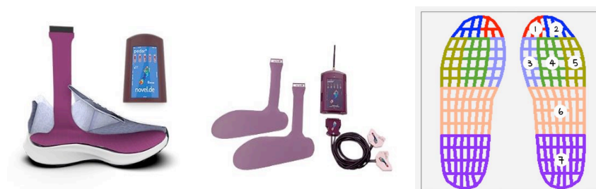
Fig. 2. In-shoe Pedar® system and seven anatomical divisions of the foot: (1) hallux, (2) lateral toe, (3) forefoot medial, (4) forefoot, (5) forefoot lateral, (6) midfoot and (7) heel.
