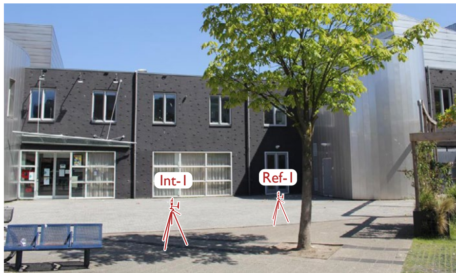
Figure 22: Example showing how to measure the effect of a solitary tree (Osdorppelein, Amsterdam).
