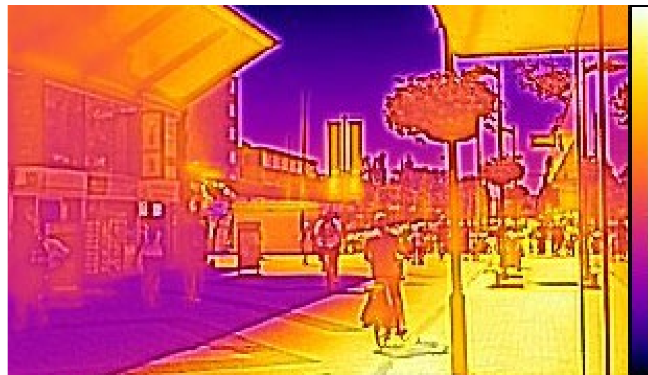
Figure 10: A thermal photograph visually demonstrating the temperature differences across Osdorppelein, Amsterdam.
