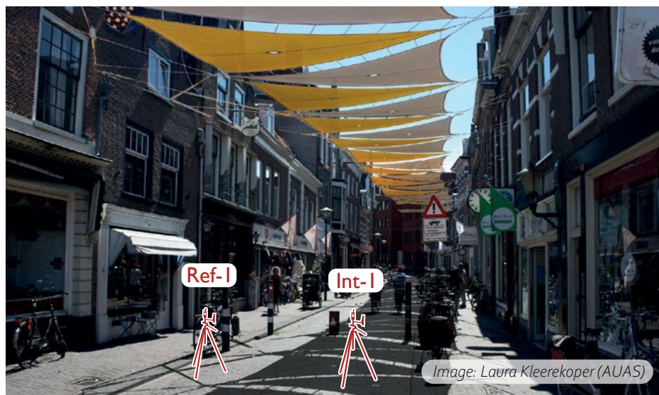
Figure 24: Example showing how to measure the effect of a shade structure (Zijlstraat, Haarlem). Adjusted image showing possible future shading scenario.
