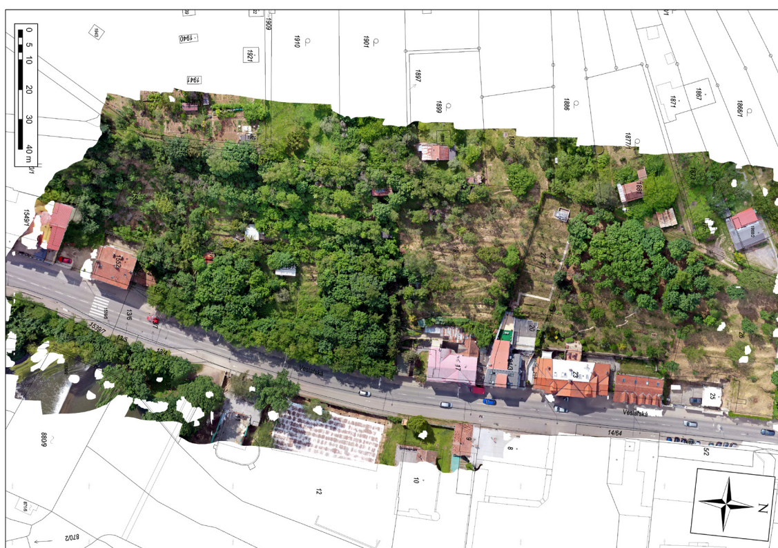
Figure 9. An ortho-photogrammetric model of the OUF site to map the site's current state and possibilities for rewilding.
