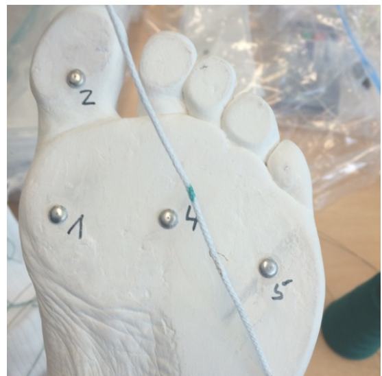
Figure 2: Temperature sensor yarn (TSY)
