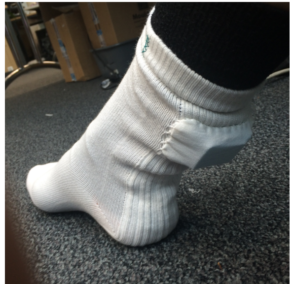
Figure 3: Temperature sensing socks developed for wear trial
