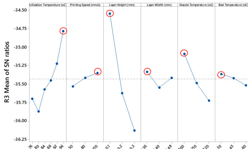
Figure 7. R3 Mean of SN ratios for each factor. Signal-to-noise: Smaller is better.
