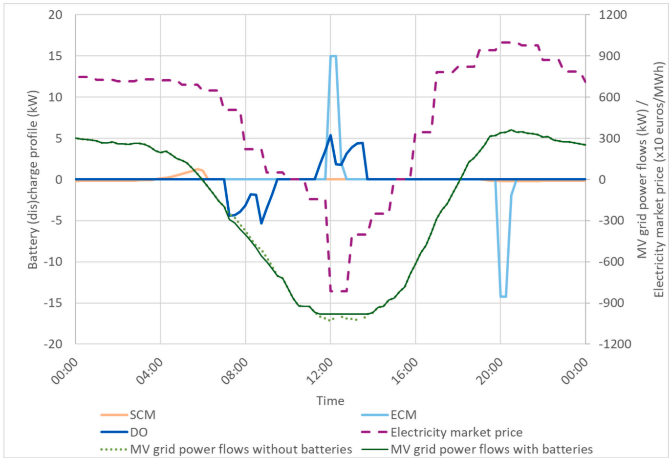
Fig. 2. Battery (dis)charge schedules for a day with high PV generation, resulting from the SCM (orange), ECM (light blue) and DO (dark blue) battery control strategies. Positive values represent battery charging and negative values represent battery discharging. For context, hourly electricity rates (purple) and MV grid power flows with (solid green line) and without (dotted green line) DO-controlled batteries are also shown. For the MV grid profile, positive values represent net consumption and negative values represent net production. Electricity market prices were multiplied by ten for clarity. (For interpretation of the references to colour in this figure legend, the reader is referred to the web version of this article.)
